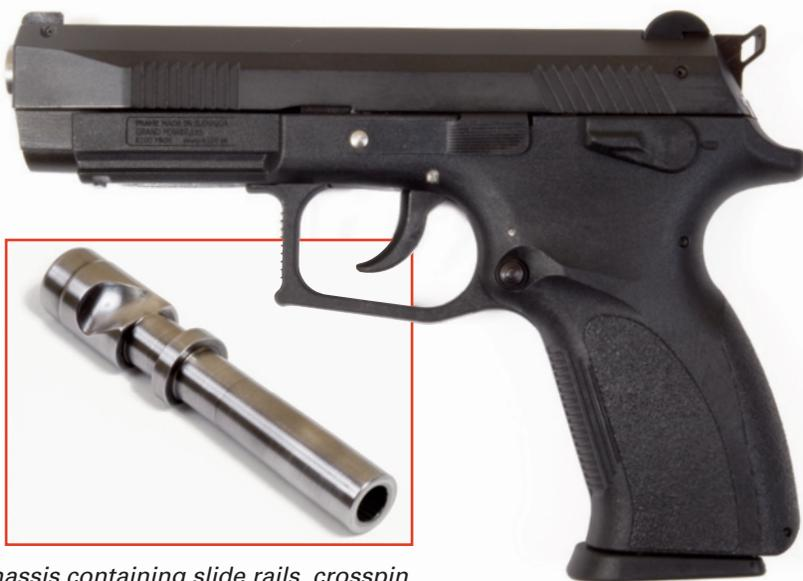
The polymer frame houses the steel chassis containing slide rails, crosspin and trigger group (l.). The crosspin engages the helical groove on the carbon-nitrided steel barrel (r.) during rotary-locked, short-recoil operation. Optimal ergonomics provide a comfortable, low-profile grip (above, r.).
